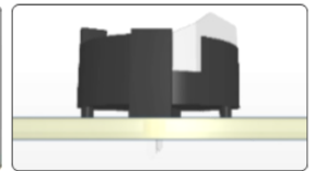
Battery socket. Notice the orientation
